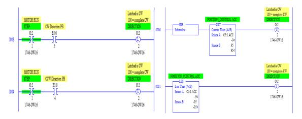
Figure 3. (a) Motor direction control (b) Oscillation mode
