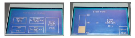
Figure 5. (a) System main menu (b) Solar panel voltage monitoring
