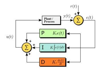
Figure 1. PID control algorithm [38]
