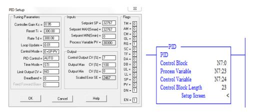
Figure 4. (a) PID setup screen, (b) PID block
